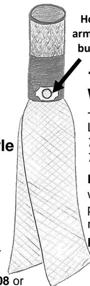
Holes in wick raiser arms attach over the 2 buttons on the sides
